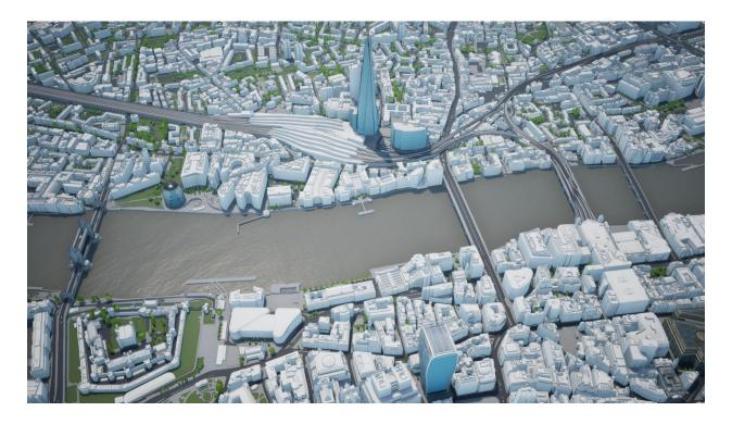
An Aerial photogrammetry 3D city model has clean geometry, high detail and up to 15 cm accuracy. Every point and every line in these 3D city models is manually captured using stereophotogrammetry. Terrain height changes are captured along features. The model is separated into layers (Buildings, Trees, Terrain layers such as Roads or Greenspaces) and is easy to update and upgrade.
