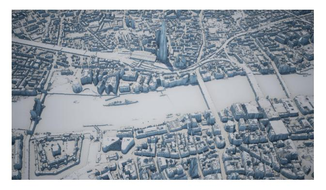
The Airborne lidar model is created by a plane collecting laser scans. Inherently a much more accurate and detailed model, great not just for backgrounds but also to measure from and even run some basic studies and simulations. Free datasets are available, just like the one by the UK Environmental agency 1m grid Lidar surveys, used in this comparison.
